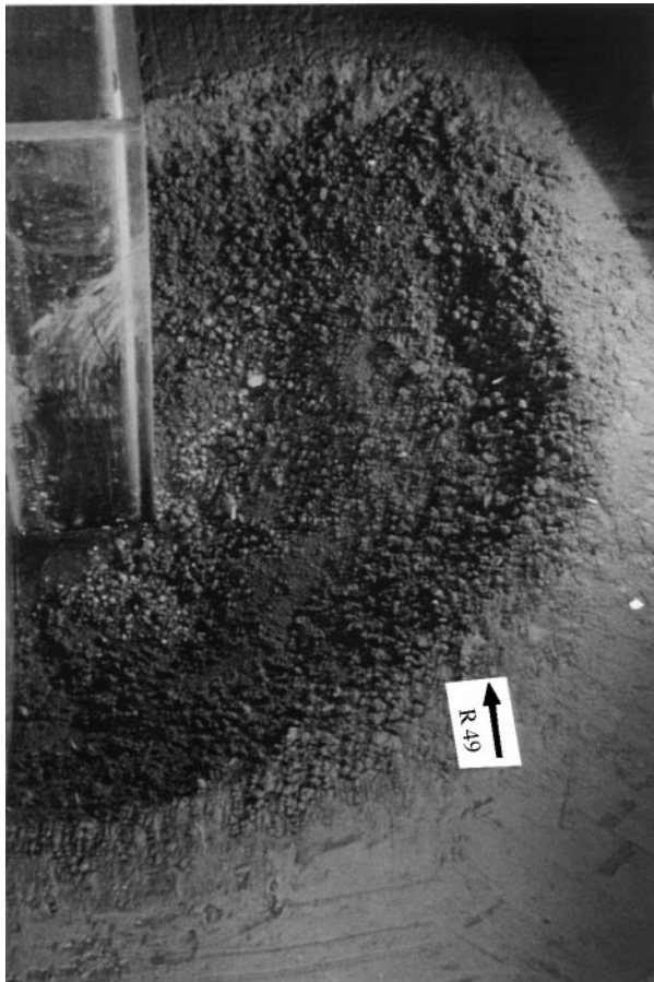
Figure 1. Local scour pattern around vertical wall abutments
